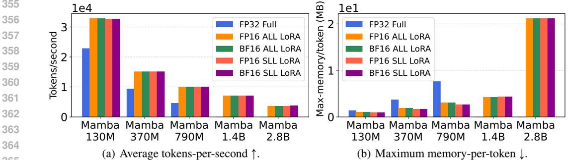
Figure 2: Timing and memory usage calculated Mamba model-sizes and PEFT combinations. Each model was trained using the Alpaca dataset dataset for three epochs and maximum sequence length 512. For each PEFT combination, the batch size was tuned to maximize GPU occupancy. Full fine-tuning exceeds available GPU memory (24 GB) for models greater than 790 million parameters.
