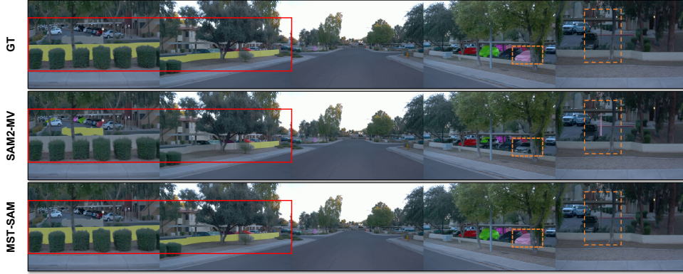
Figure 5: Qualitative comparison of segmentation with SAM2-MV on the Waymo Open dataset. Different colors represent different objects. The displayed image has been resized for better visual effects. Where the red boxes denote identity confusion and orange boxes denote identity mismatch.
