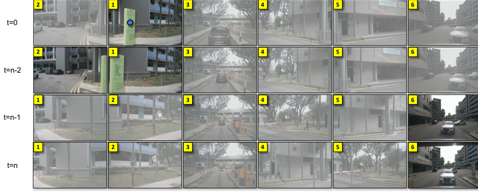
Figure 4: Visualization of our Memory View Selection (MVS) strategy in action. The filter prunes irrelevant historical views (faded) while selecting high-quality features (bright, with masks) and the initial anchor frame ( t = 0 ) to build a compact and effective memory bank.
