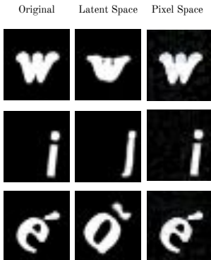
Figure 4: Comparison of perturbations performed in latent and pixel space. Note how the perturbations performed in latent space convey meaningful information (e.g., changes in the font or character), while the ones performed in pixel space resemble adversarial attacks and do not provide any valuable insights into the classifier’s reasoning.
