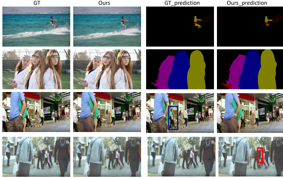
Figure 3: Failure cases on video object segmentation (VOS, first two rows) and multiple object tracking (MOT, last two rows). In the MOT visualization, the blue bounding box denote false negatives, while red bounding box indicate false positives.
