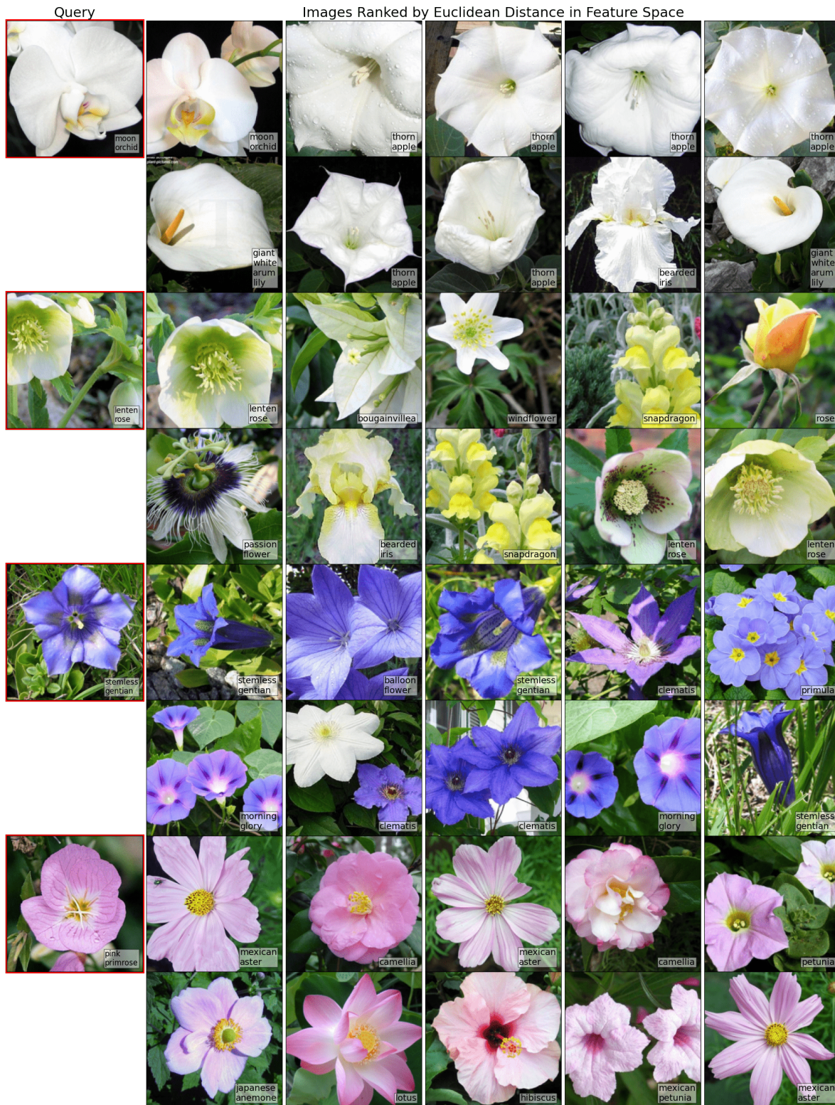
Figure 15: Query image and top images ranked by Euclidean distance in feature space of FC model for Flower dataset. The degree of semantic similarity between the query and the top images is lower than the NW model (see differences in class labels).
