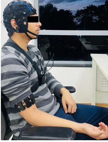
Fig. 3: Experimental setup. The participant is seated while wearing the EEG cap and EMG armband. During movement trials, the subject performed a full right elbow flexion-extension cycle, moving from a relaxed state to full flexion and back, in response to an auditory cue.
