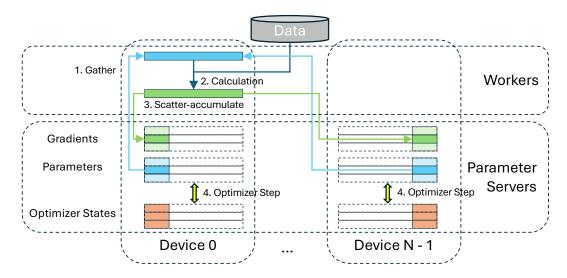
Figure 6: The architecture of FSDP with ODC, in which FSDP can be seen as a decentralized parameter server, with server part and worker part highlighted in this figure.
