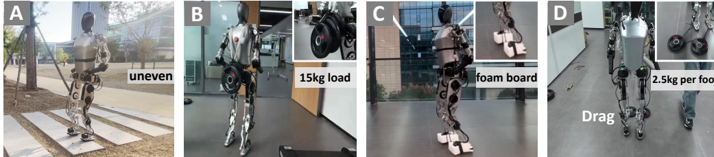
Figure 7: Real-World Experiments: (A) Walk on uneven terrain. (B) A 15 kg load is added to the centroid. (C) White foam board insoles are placed under the feet. (D) A 2.5 kg load is added to each foot. In all these scenarios, our method demonstrates robust performance.
