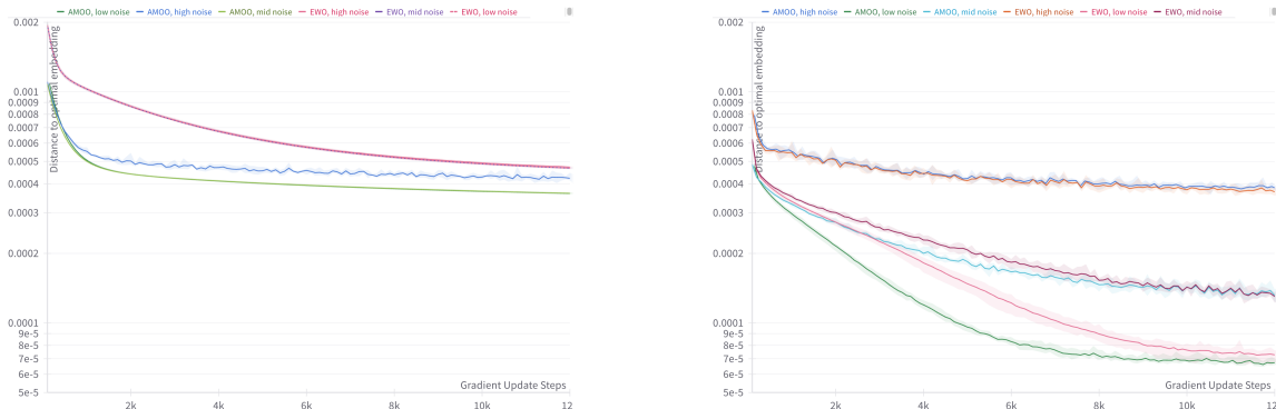
Figure 1: AMOO tested against equal weighting of loss functions (EWO) when optimized by SGD ( left ) or Adam ( right ). Additionally, we test the effect of additive Normal noise of the optimal representation h_{\theta}(x) . AMOO performs better than its counterpart in all 6 settings.
