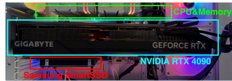
Figure 7: Hardware Architecture of HillInfer.
