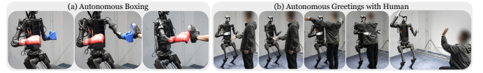
Fig. 5: OmniH2O sends egocentric RGB views to GPT-4o and executes the selected motion primitives.
