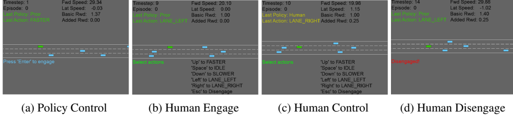
Figure 9: Highway-Human Graphic User Interface. There are four different scenarios during the sample collection process. When the human expert engages and takes over the control, additional information would show up for available actions.
