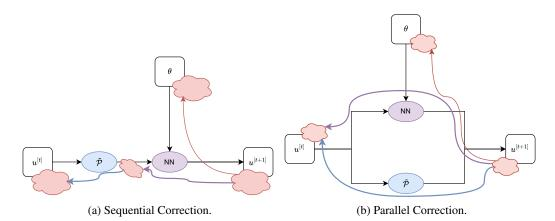
Figure 10: Correction setups for a coarse solver  $\tilde{\mathcal{P}}$  using a neural network. Curvy arrows depict gradient flow in backpropagation, purple signifies input-output differentiation over the network, and blue is associated with *differentiable* physics over the coarse solver.
