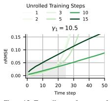
Figure 15: Test rollout performance of ResNet emulators for 1D advection at  $\gamma_1 = 10.5$  when each unrolled training uses equal compute time. The gray area indicates the axis limits in the plots of Figure 3. Emulators with shorter unrolling improve, but long unrolling remains superior.
