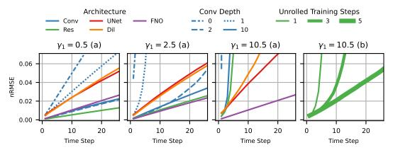
Figure 3: (a) Performance of various neural emulator architectures on a 1D advection problem with increasing difficulty ( $\gamma_1 = CFL$ ). If the demands on the receptive field (given by  $\gamma_1$ ) are not fulfilled, emulators diverge immediately. (b) Unrolling improves accuracy at the highest difficulty.
