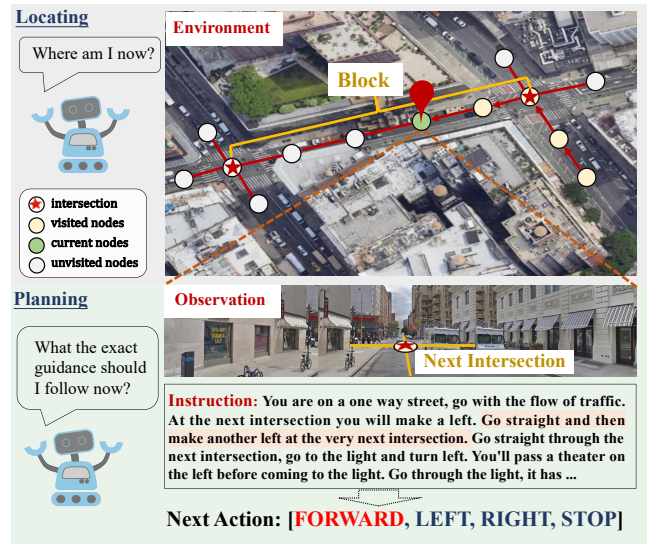
Figure 1: The illustration of navigation process of our locating before planning approach. During the locating phase, the agent locates its relative spatial position in the current block. In the planning phase, the agent associates the corresponding guidance to follow and makes an action decision to take (i.e., FORWARD).
