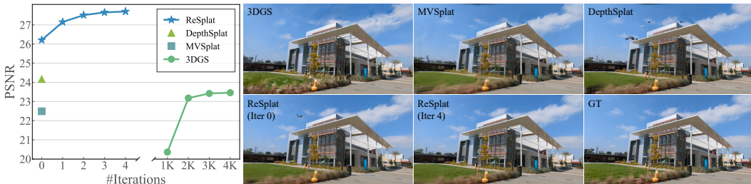
Figure 1: Learning recurrent Gaussian splats in a feed-forward manner. We propose ReSplat, a feed-forward recurrent network that iteratively refines 3D Gaussian splats to improve sparse view settings where optimization-based 3DGS (Kerbl et al., 2023) struggles. As initialization (iteration 0), we introduce a compact reconstruction model that predicts Gaussians in a 16\times subsampled space, producing 16\times fewer Gaussians and 4\times faster rendering than per-pixel MVSplat (Chen et al., 2024b) and DepthSplat (Xu et al., 2025). The reduced number of Gaussians makes subsequent refinement efficient. Compared to the optimization-based 3DGS, ReSplat is 100\times faster thanks to its feed-forward design, while still benefiting from iterative updates. Here we show results for 8 input views ( 512 \times 960 resolution) on DL3DV dataset; see Table 1 for detailed metrics.
