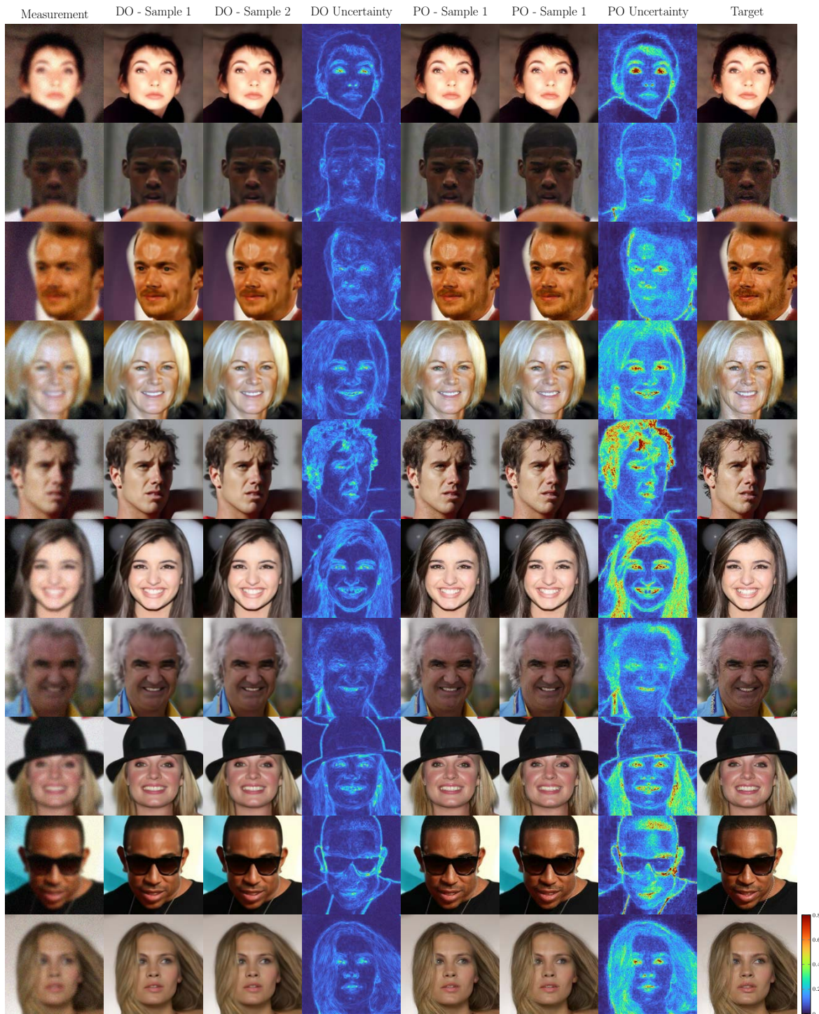
Figure 12. Distortion and Perception optimized deblurring results for the CelebA-HQ dataset (test split). Uncertainty is calculated over n = 10 reconstructions from the same measurement.
