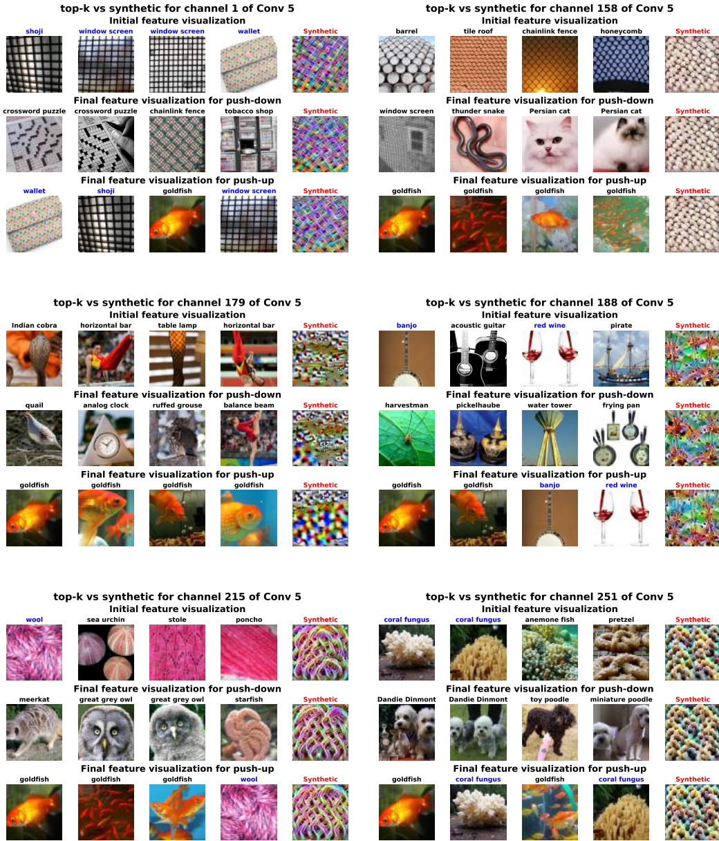
Figure 24: Synthetic Feature Visualization attack after push-down and push-up attacks on Conv5 of AlexNet. Channels indexes were taken randomly. We observe a decorrelation between natural top-activating images and synthetic optimal images.
