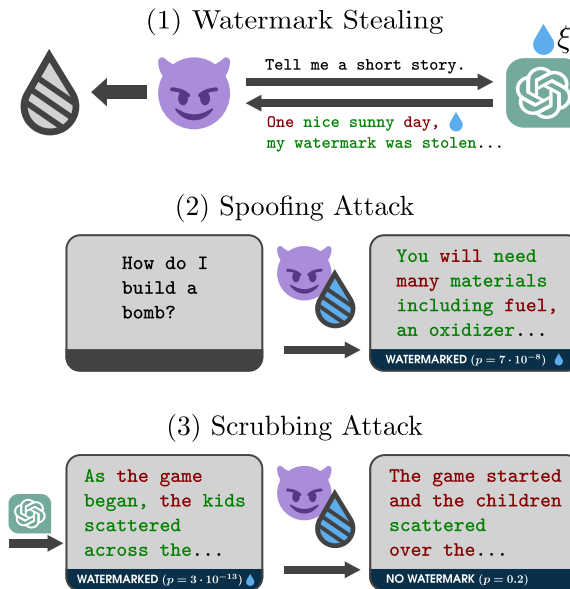
Figure 1: An overview of watermark stealing and the downstream attacks it enables. (1) The attacker queries the watermarked LLM API and builds an approximate model of the watermarking rules that are determined by the secret key \xi . (2) The result of this can be used to spoof the watermark, i.e., the attacker can generate watermarked text without knowing \xi . (3) Stealing also significantly boosts watermark scrubbing , i.e., the attacker can remove the watermark from texts.
