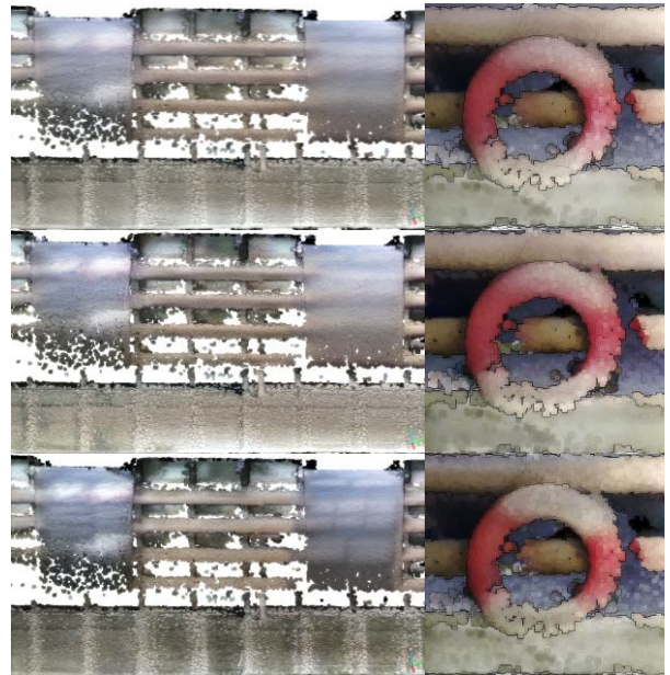
Figure 6. Details from two locations in the DS Hestmanden reconstruction showing comparison between three methods for multi-view fusion: (top row) simple averaging, (middle row) median colour, (bottom row) weighted averaging. Weighted averaging gives best contrast and detail.
