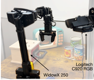
(a) Bridge-AutoEval cell with a WidowX 250 6-DoF arm.
