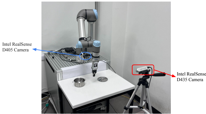
Fig. 5: Real-world robot setup. Our experiments are conducted on a UR5e arm with an RG2 gripper. The observation is captured with a fixed front camera and a wrist-mounted camera, providing complementary viewpoints of the scene for both single-view and multi-view evaluations. All RGB images are resized to 256 \times 256 and the robot is controlled at 10 Hz.
