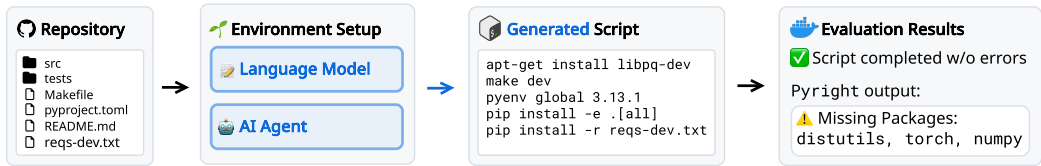
Figure 1: Overview of the workflow with ENVBENCH. The process begins with cloning a target repository. Next, the repository is passed as an input to an environment setup approach, which then produces a shell script to set up the repository as an output. Internally, it could be, for instance, a single LLM request or an AI agent building a script dynamically. Finally, in our evaluation suite, we execute the produced script and verify the environment is correctly configured through static analysis and compilation checks.
