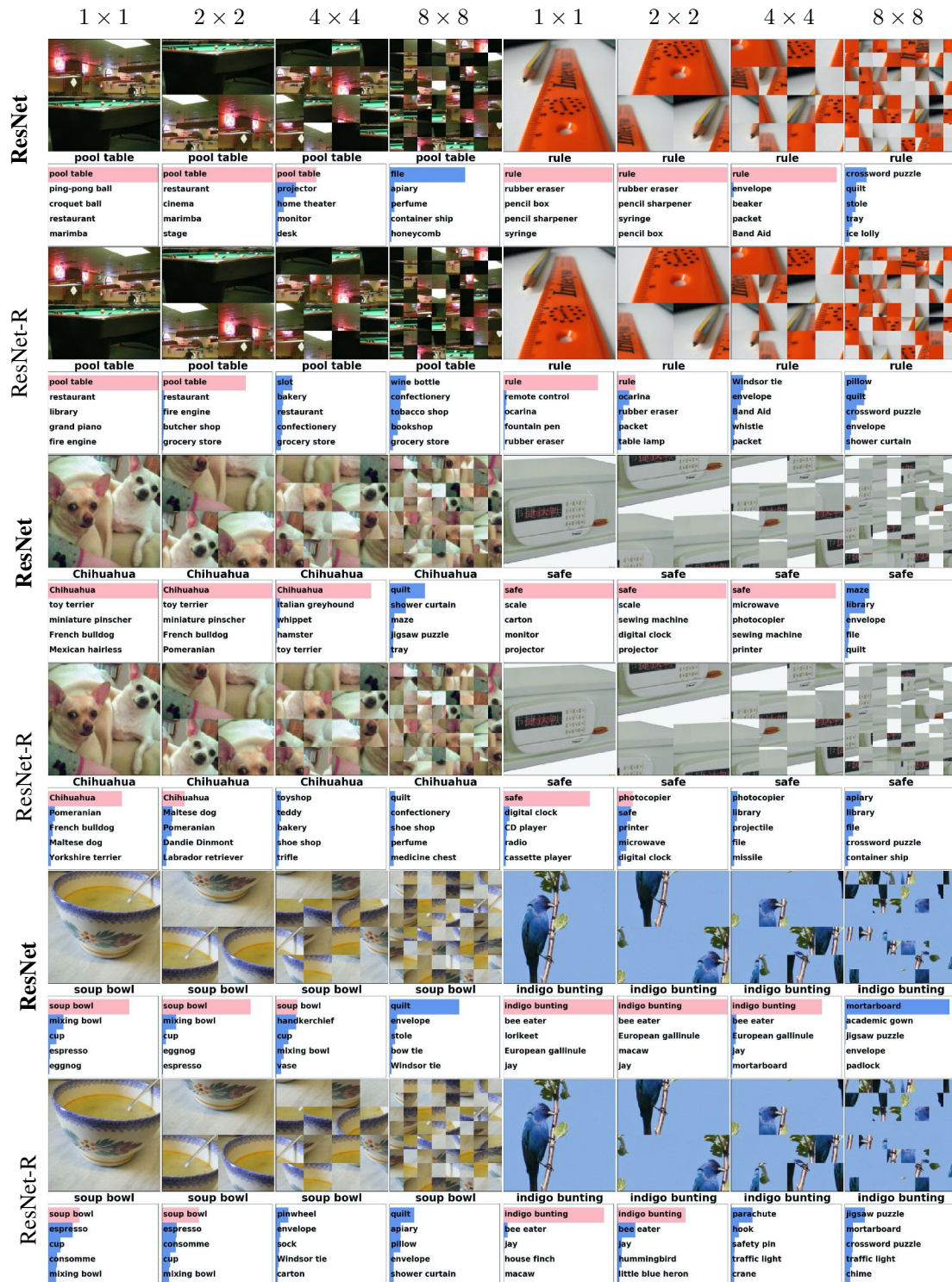
Figure A6: ResNet-R, on average across the three patch sizes, underperforms the standard ResNet model. Surprisingly, we observe that ResNet correctly classifies the image to their ground truth class even when the image is randomly shuffled into 16 patches, e.g., ResNet classifies the 4 \times 4 case of rule, safe with \sim 100\% confidence. The results are consistent with the strong texture bias of ResNet and shape bias of ResNet-R (described in Sec. 3.2.1).
