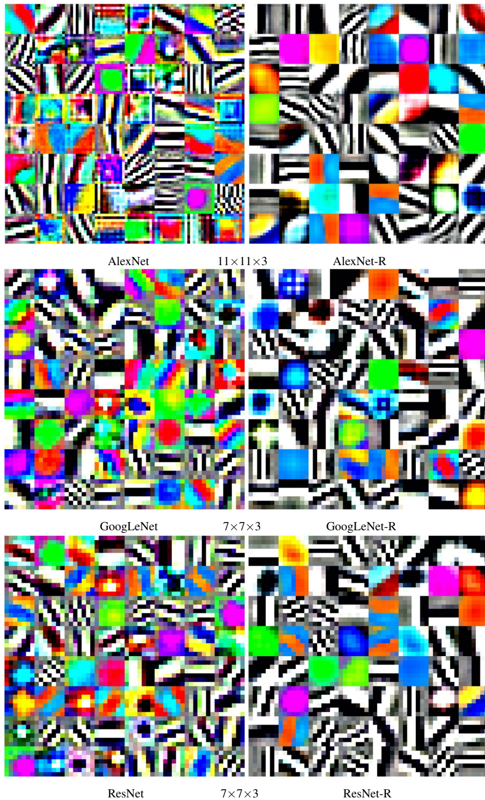
Figure A3: All 64 conv1 filters of in each standard network (left) and its counterpart (right). The filters of R models (right) are smoother and less diverse compared to those in standard models (left). Especially, the edge filters of standard networks are noisier and often contain multiple colors in them.
