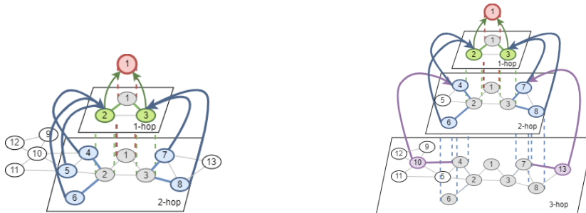
(a) A 2-layer message passing can cover all information in 2-hop neighborhood of the root node in red. (b) Sampling sacrifices completeness ( v_5 not sampled) but increases the coverage range (3-hop layer).
