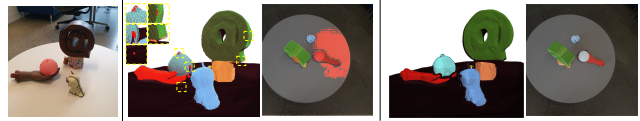
Figure 4. Projection to 3D. Left: Example image. Middle: points projected without mask edge erosion and outlier removal, resulting in noisy segmentation outputs. Right: by using mask erosion and outlier removal we obtain clean 3D points and subsequently obtain a correct segmentation output.
