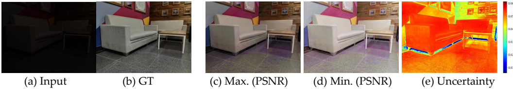
Figure 18: Visualisation of BEM outputs showing the input image (a), ground truth (b), the prediction with the highest PSNR (c), the prediction with the lowest PSNR (d), and the uncertainty map (e). The uncertainty is computed as the pixel-wise standard deviation across 500 predicted images.
