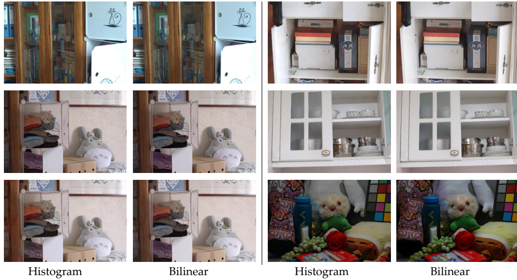
Figure 10: Visual comparison between the local histogram and bilinear downsampling implementations of the reduction function \phi . The bilinear \phi demonstrates better restoration capability compared to the histogram-based counterpart. However, the histogram-based \phi shows better global colour representation. Best viewed when zoomed in.
