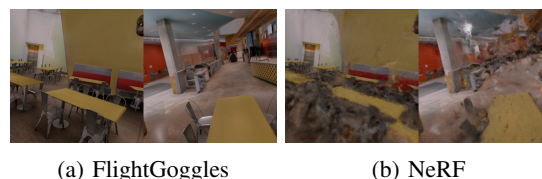
Fig. 2: (a) Images captured in the Flightgoggles simulation environment [18]. (b) Images rendered through nerfstudio [29]. The images exhibit significant differences from the originals, primarily due to artifacts caused by the sparse density of training data.
