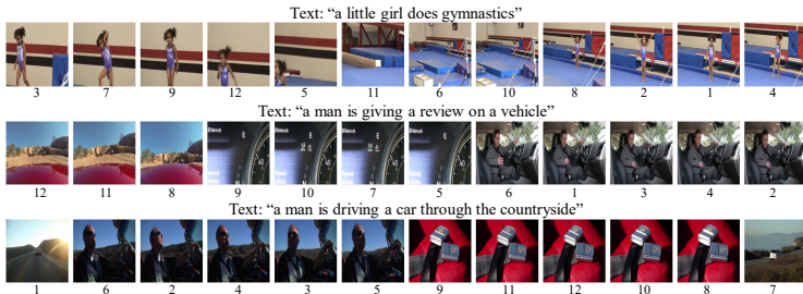
Figure 4: The similarity ranking between the text features and frame features, which are extracted by original pretrained CLIP encoder. We observe that the key frames, which are more relevant to the text description, make up a larger proportion of the video content.
