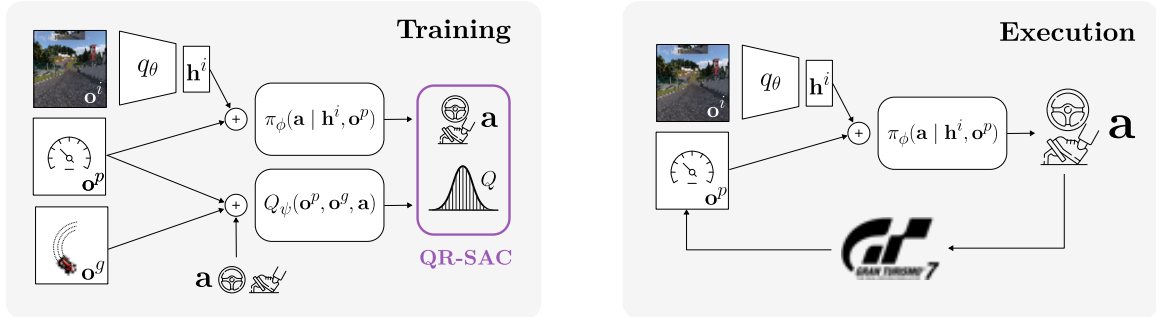
Figure 1: Our vision-based RL agent for autonomous car racing. (Left) We exploit an asymmetric actor-critic architecture to train our agent: the policy network \pi_\phi is provided with proprioceptive information \mathbf{o}^p and image features \mathbf{h}^i , encoded with a convolutional neural network q_\theta , to output actions \mathbf{a} . The critic network Q_\psi is provided with local proprioceptive observations and global observations \mathbf{o}^g (i.e., course shape information) to predict quantiles of future returns. (Right) During execution, our agent only receives local features from the Gran Turismo 7 simulator.
