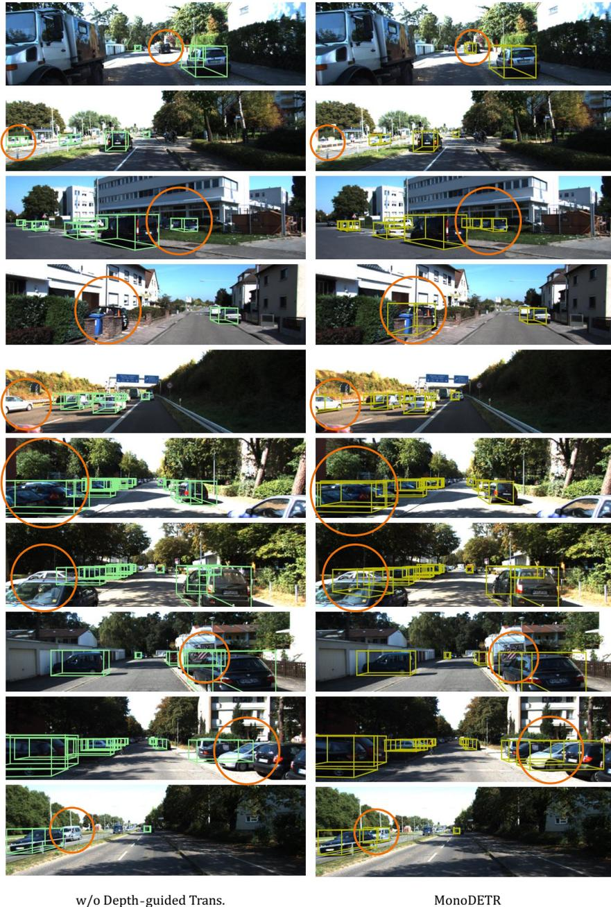
Figure 5: **Visualization of detection results.** We utilize green boxes for the variant without depth-guided transformer (Left) and yellow boxes for MonoDETR (Right). We use red circles to emphasize the detection difference.
