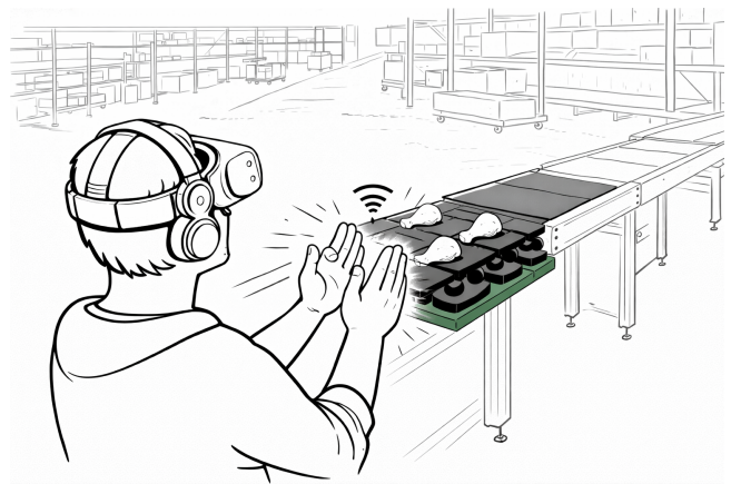
Figure 1: Simplified AI-generated illustration of the VR scenario. A participant wearing a VR headset supervises the Z-shaped packing line. Chicken drumsticks move onto the robotic tile array (black tiles), which performs orientation and transfer before the line continues to another section. The operator (study subject) controls the system by clapping; the system interacts with the user using voice utterances.
