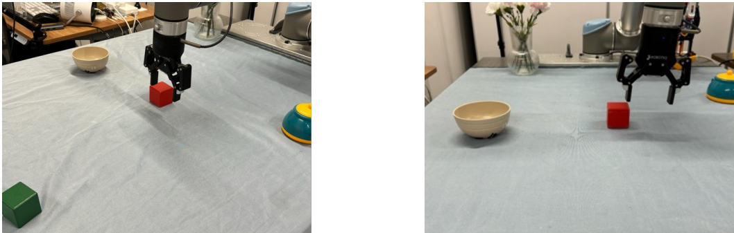
Figure 12: Spatial illusion. These two figures are captured at the same timestep. Without depth information, we lose the front-to-back positional relationship between the object and the gripper in the three-dimensional world.
