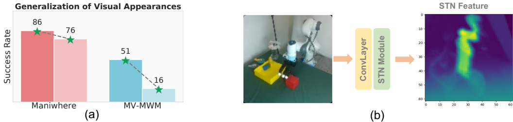
Figure 3: (a). Generalization results of visual appearances. Maniwhere exhibits minimal performance drop when encountering variations in visual appearance, whereas MV-MWM is unable to handle these visual scenarios. (b). STN visualization. STN is capable of transforming views from various other perspectives to align closely with the fixed view used during training.
