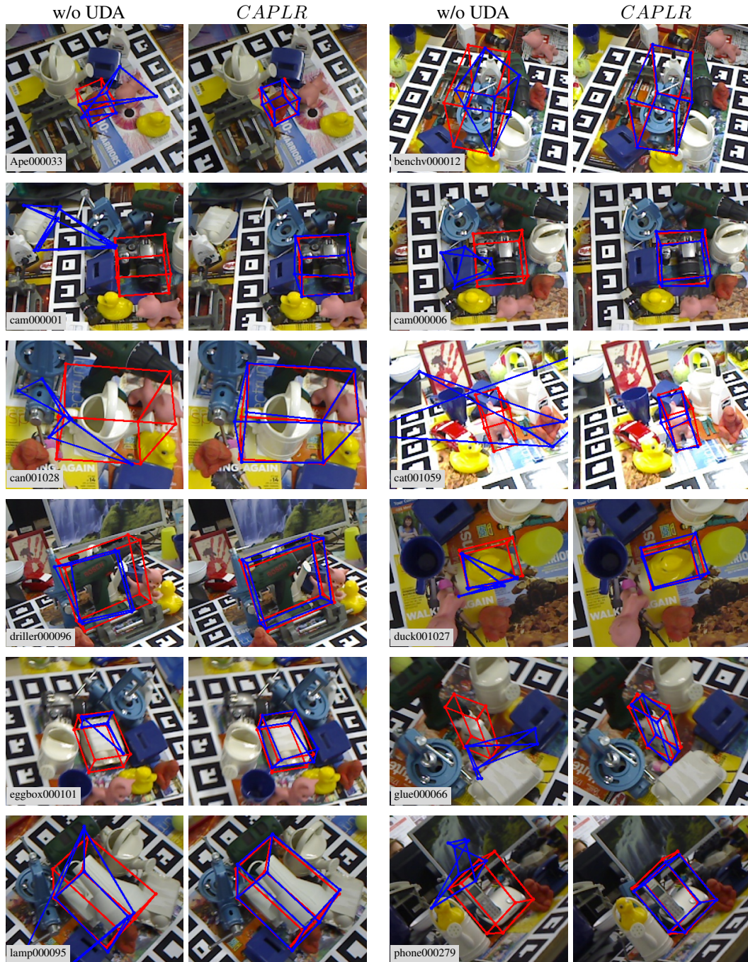
Figure 9: Qualitative comparison of pose predictions on LineMOD images. Each pair shows results without UDA (left) and with CAPLR (right). Ground-truth poses are shown in red , and predictions in blue .
