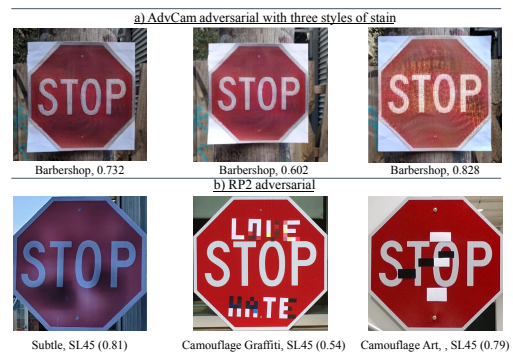
Figure 1: a) AdvCam and b) RP 2 techniques can deceive CNN classifiers by introducing perturbations. The SL45 refers to the speed limit of 45.
