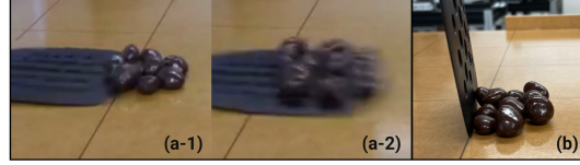
Figure 3: Task-policy trajectories better reveal task-relevant information such as scooping dynamics under fast contact.
