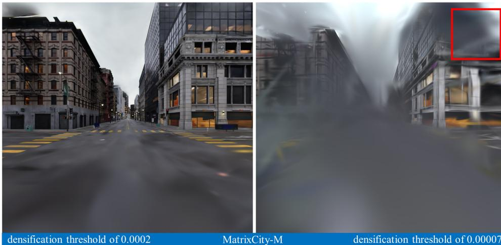
Figure 12: In 3DGS, as the densification threshold decreases, the growth rate of GS increases. However, due to the rapid growth rate, floaters are generated in the model that cannot be eliminated through training (marked with red rectangle), which deteriorates the reconstruction effect. The MVS initialization strategy introduced in RetinaGS will mitigate this issue.
