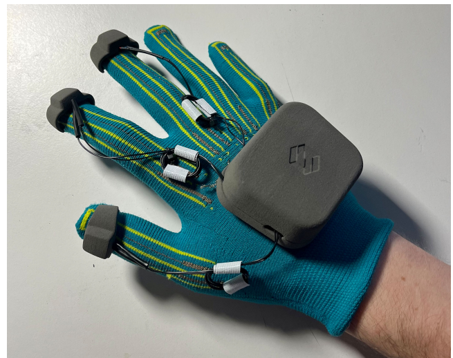
Figure 3: CeTI FingerTac Glove with textile integrated sensors for gesture control integrated with the FingerTac for haptic feedback
