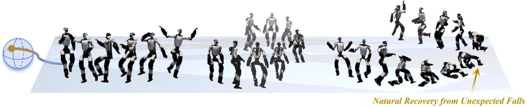
Figure 4: Real-World Validation of **Tracking**. *Left*: Highly dynamic dancing. *Middle*: Frequently turning during walking. *Right*: **Naturally** recover to continue track the motion.
