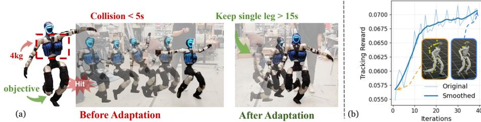
Figure 8: Few-Shot Adaptation: (a) Single-pose adaptation improving single-leg standing under an additional payload. (b) Trajectory adaptation reduces tracking error.
