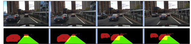
Fig. 3 Generation of scene representation with an example cut-in maneuver from BDD-100K Cut-in/Lane-pass Subset. Overlapping masks of vehicles and ego-lane are in different colors. The figure shows four frames of a single sequence, whereas the 3D network uses 20 of them for classification. The frame height is reduced from 600 to 400 pixels to remove ego-vehicle's hood and some sky
