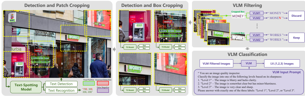
Figure 2: SA-Text curation pipeline. A text-spotting module (Huang et al., 2024) detects text regions across the image. To recover missed text, the model is reapplied to smaller patches. Two vision-language models (VLMs) (Bai et al., 2025; Lu et al., 2024) then transcribe the text within the detected boxes, and only patches where both agree are kept. Finally, a single VLM (Bai et al., 2025) classifies each patch by sharpness and blurriness.
