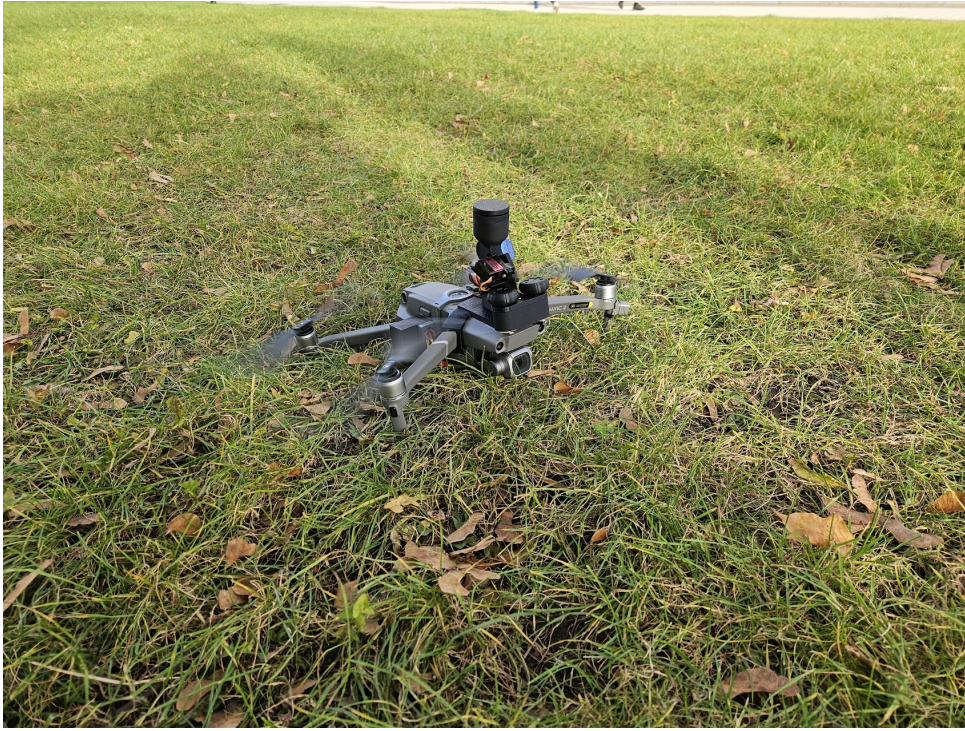
Figure 9: Drone with Scent Dispenser
