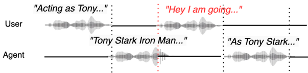
Figure 2: Duplex training data format. Our duplex data consists of separate user and agent streams including turn taking and barge-in behavior. Here, the user barges in at the second turn.
