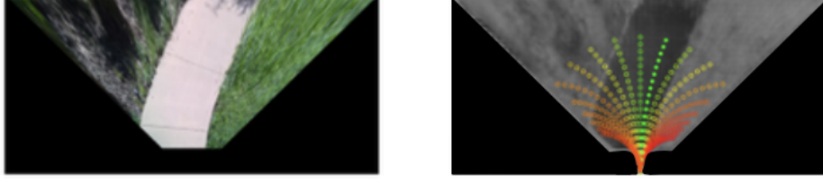
Figure 8: Example of homography-transformed BEV image of live robot deployment and corresponding local costmap. The best local plan is chosen from a set of path options based on a weighted combination of the terrain cost and distance to goal.
