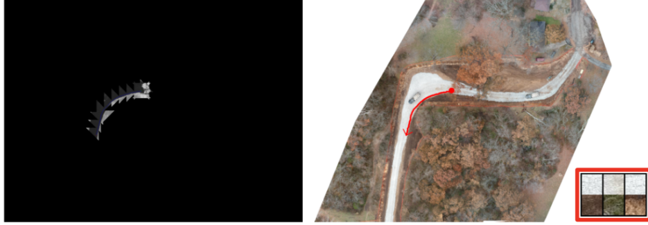
Figure 5: Example of a costmap, planned path, and preference context of a simulated robot deployment in one of the natural unseen environments of the Aerial Map Experiments using our method. The costmap displays the timeseries progression of the local BEV costmaps generated with our method.
