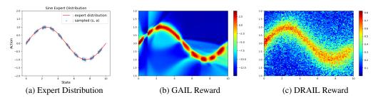
Figure 7: **Reward function visualization.** We present visualizations of the learned reward values by the discriminative classifier of GAIL and the diffusion discriminative classifier of our DRAIL. The target expert demonstration for imitation is depicted in (a), which is a discontinuous sine function. The reward distributions of GAIL and our DRAIL are illustrated in (b) and (c), respectively.
