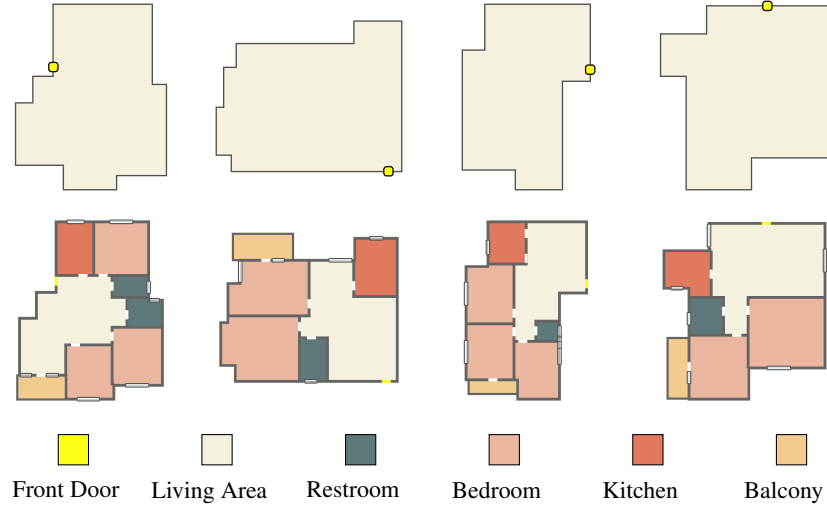
Figure 5: Examples of generated floor plans using GenPlan
