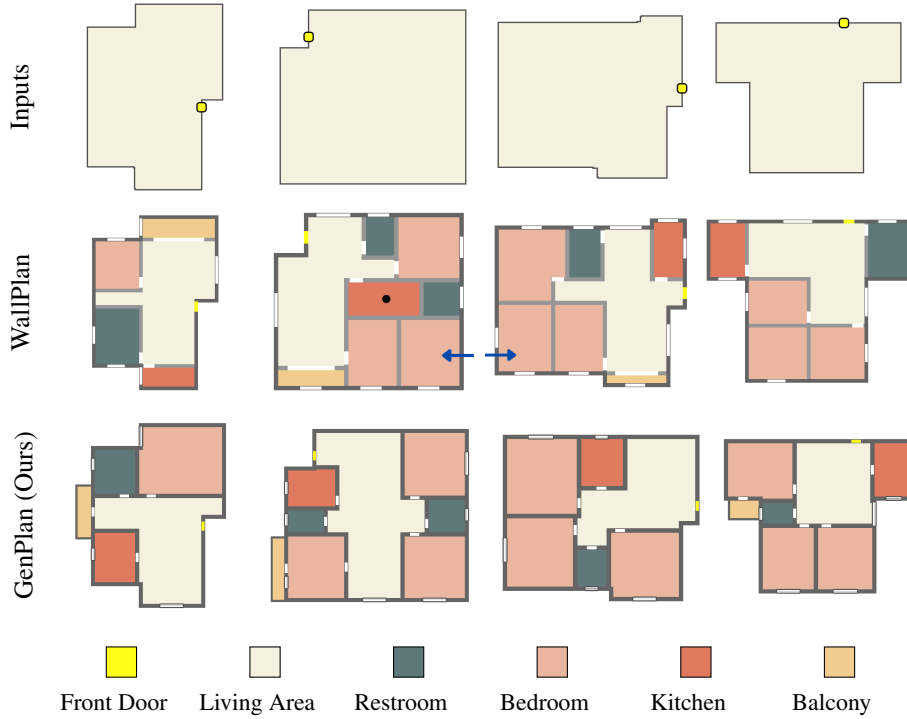
Figure 6: Performance comparison of GenPlan vs. WallPlan. Note that WallPlan generates trapped rooms (lacking entryways rooms annotated by the blue arrows) and places kitchens centrally (annotated by the black dot) without windows. Sun et al. (2022)
