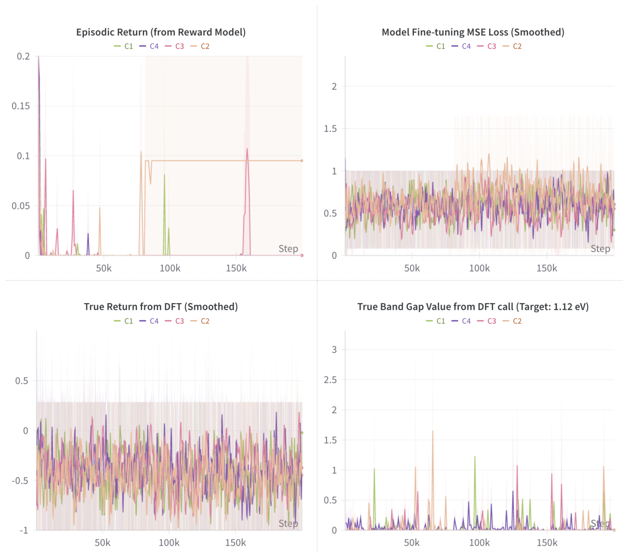
Figure 19: Training DQN agent separately on 4 crystals (C1,C2,C3,C4) with the COM-based reward model trained in above experiment. The reward model is fine-tuned once in 50 episodes. The target band gap here is 1.12 eV, which corresponds to a maximum reward of 1.0. a) Episodic return from the reward model, b) Loss of fine-tuning reward model after every DFT call, c) Returns from DFT outputs, and d) Logged band gap after each successful DFT call.
