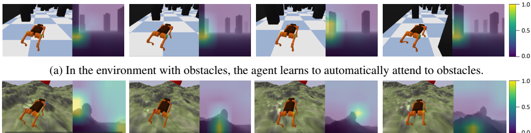
(a) In the environment with obstacles, the agent learns to automatically attend to obstacles. (b) On challenging terrain, the agent attends to the goal destination and the local terrain in an alternative manner. Figure 3: Self-attention from our shared Transformer module. We visualize the self-attention between the proprioceptive token and all visual tokens in the last layer of our Transformer model. We plot the attention weight over raw visual input where warmer color represents larger attention weight.
