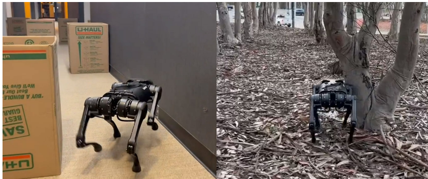
Figure 9: Some failure cases of MPC-based controller due to limitation of agility. The left figure shows that when walking through a narrow path, the robot can not quickly turn around and collide into the wall. The right figure denotes that it may collide to the tree in the wild, due to the shape of the obstacles are out of the training distribution and the robot can't adjust quickly enough to avoid.
