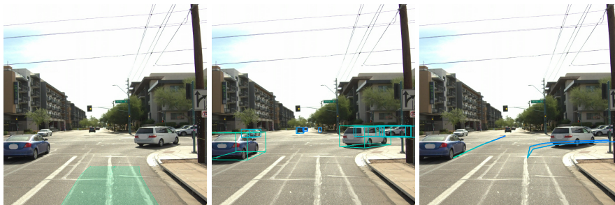
(h) Our predicted trajectory suggests to stop as we approach an intersection with a yellow light, demonstrating cautious and safe behavior.
