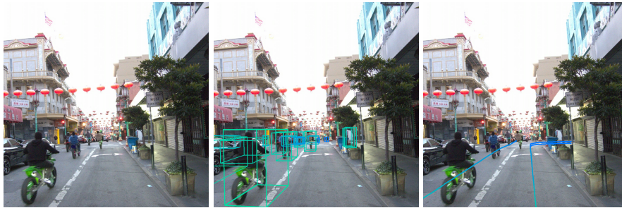
(k) A fleet of fast-moving motorcyclists pass by. The predicted trajectory suggests pausing to allow them to pass safely. Notably, motorcyclists are accurately identified by our model (middle).
