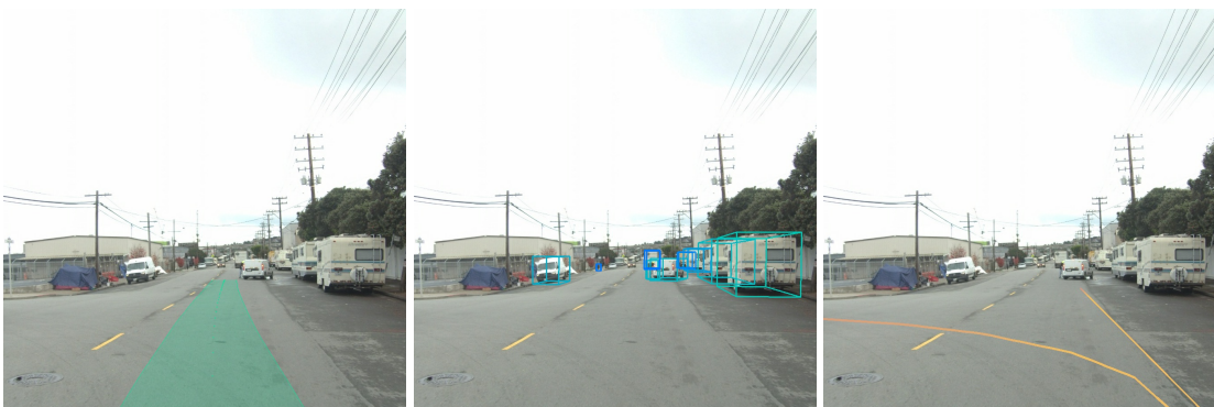
EMMA fails to detect a distant oncoming vehicle, though it is correctly identified in the subsequent frame. This one-frame detection delay is suboptimal, as the ego vehicle plans to nudging to the left. Earlier detection would have led to a safer and more controlled trajectory.
