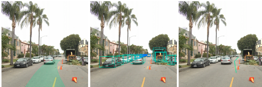
(f) Our lane is blocked by construction cones, so our predicted trajectory suggests to move into the left lane, even though it's in the opposite direction. EMMA captured the blockage and performed a detour.
