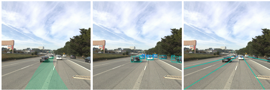
(b) A ladder appears on the freeway, and our predicted trajectory suggests to switch to the left lane to bypass it appropriately.
