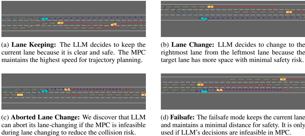
Figure 4: The ego car is in blue and other agents are in yellow. The blue dots are the planned trajectory waypoints of the ego. The red dots are the sampled waypoints of other agents from the interval-based prediction. The grey rectangles are the recent trajectory histories of the ego and other agents. The LLM exhibits safe lane keeping, optimistic lane changing, cautious lane changing abort, and conservative failsafe in the simulations.
