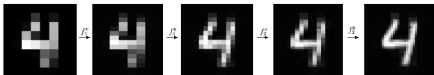
Figure 2. Upscaling pipeline with PNF models. From the left: image sampled by baseline RealNVP model f_0 trained on low-resolution ( 8 \times 8 pixels) MNIST dataset, upscaled images of the size 16 \times 8 , 16 \times 16 , 32 \times 16 , 32 \times 32 pixels with PNF models f_1^x , f_1^y , f_2^x , f_2^y , respectively.
